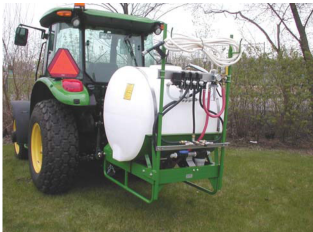
Boomless nozzles are ideal for rough ground, pastures, prairie and right-of-way areas.
